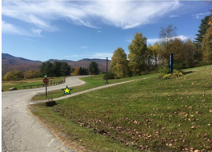
**Figure 8. A grass swale transports stormwater to the intersection with College Hill where a bioretention practice is proposed (shown with a star).**
