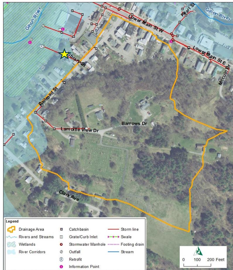
**Figure 10. The drainage area for the proposed BMP is shown in orange for the Railroad St site. The proposed BMP location is in the Town Library parking lot along Railroad St, which is shown with a star.**
