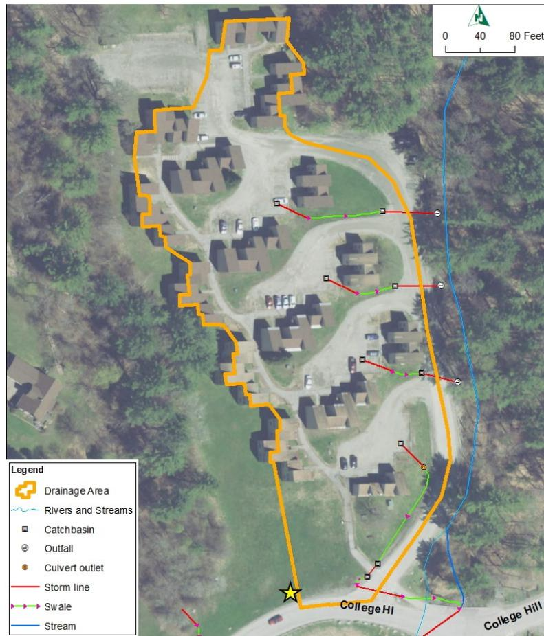
**Figure 11. The drainage area for the proposed BMP is shown in orange. The proposed BMP location is shown with a star.**
